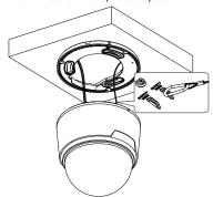
Attach the camera body to the install mount. Turn the camera body clockwise to fasten.
