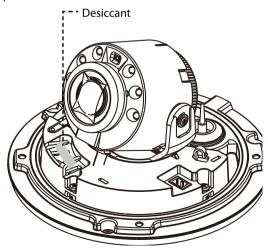
6 Use the screws, anchor provided with the camera to secure the install body on a wall or a ceiling.
