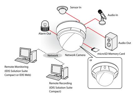
Control the camera over the network from software installed on a computer. Ideal for using the camera over the network from a remote location.
