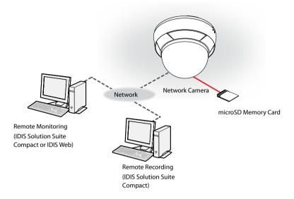
Control the camera over the network from software installed on a computer. Ideal for using the camera over the network from a remote location.
