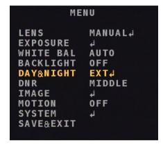
EXT: The light sensor automatically switches the COLOR and B&W mode.
