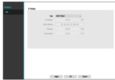
DHCP Client: Retrieves an IP address and other network settings automatically from a DHCP server.
