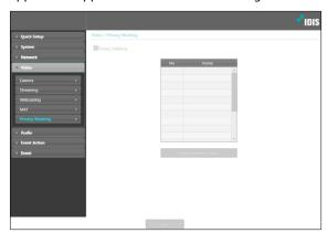
Privacy Masking Setup: Set up privacy masks (up to 8). Privacy masks are set up on Original View video. Thus, if video is dewarped, privacy masks are also dewarped.
