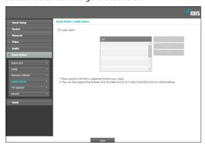
List: Displays a list of audio files to playback. Click Add or Remove to add/remove audio files. Select an audio file from the list and then click Play to listen to the file. The total audio file upload capacity is 10MB.
