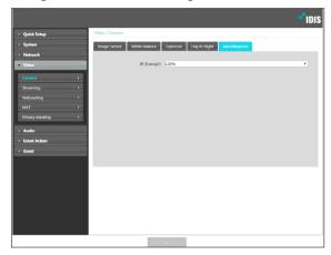
• **IR Strength:** Set the brightness of the IR LED. The higher the value is set, the brighter it is.
