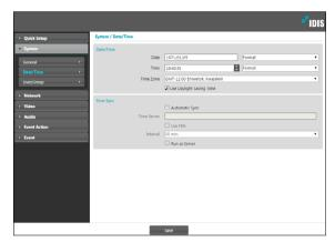
Date/Time: Change the camera's date/time settings and display formats and configure the time zone and daylight saving time settings. Click Save to apply the changes right away.
