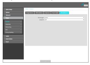
**IR Strength:** Set the brightness of the IR LED. The higher the value is set, the brighter it is.
