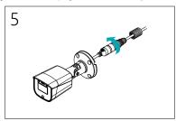
Push the waterproof cap body and cap into the RJ45 jack and rotate it.
