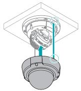
2 Fasten the screws for the dome cover clockwise using the allen wrench.
