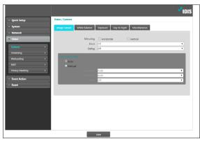
• **Mirroring**: Select Horizontal Reverse or Vertical Reverse to flip the image horizontally or vertically.
