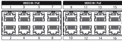
Connect network cameras or video encoders to the NVR using RJ-45 cable (Cat5e, or Cat6). In addition to cameras or video encoders, you can connect external hubs (Optional: DH-2112PF, DH-2128PF) to form a network. The NVR recognizes DirectIP™ network cameras automatically. Ports 1 through 16 support PoE.
