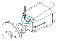
2 Insert a SD memory card into the SD memory card slot with the 'micro SD' print facing upward.
