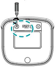
Make sure that the cover is joined properly when screwing it; otherwise, the IP67 level is not quaranteed.
