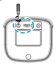
Insert a SD memory card into the SD memory card slot with the 'micro SD' print facing upward.
