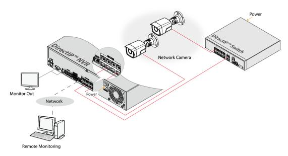
DirectIP $^{\text{TM}}$  NVR makes it easy to use cameras without extra network configurations. Each camera can be controlled via the DirectIP $^{\text{TM}}$  NVR setup menu, without any PC. For detailed camera settings, please see the camera setting pages of DirectIP $^{\text{TM}}$  NVR manual.
