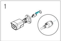
1 Insert a round rubber ring (silicone rubber) into the RJ45 jack.
