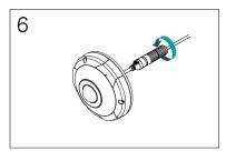
Lock the waterproof cap into the waterproof cap body.
