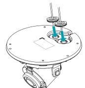
5 Attach the enclosed desiccant in the bottom to prevent moisture.
