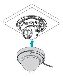
Remove the protective film inside and outside before closing the dome cover.
