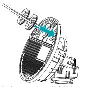
5 Use the screws, anchor provided with the camera to secure the bottom cover on a wall or a ceiling.
