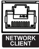
This NVR is capable of connecting to networks via an ethernet connector. Connect an RJ-45 cable (Cat5, Cat5e, or Cat6) to the NVR's network port. It's possible to operate and upgrade the NVR remotely over a network. For more information on ethernet connection setup, refer to **Network Setup in the operation manual**.
