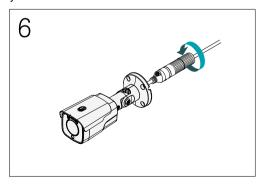
6 Lock the waterproof cap into the waterproof cap
