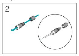
Insert the network cable into the waterproof cap, rubber bushing, and waterproof cap body in order.
