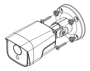
Screw the mounting bracket to the wall or ceiling by using screws(4) and bushings(4) provided with the camera. Adjust the camera angle by bending the stand. After fully assembling the joint screws, unscrew it 2 ~ 2.5 turns again and move the cover of the joints of the left 3 places slightly. (The screws should not be completely released to prevent it from falling.) After adjusting the direction of the camera, turn the screw clockwise to secure it completely.
