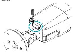
Insert a SD memory card into the SD memory card slot with the 'micro SD' print facing upward.
