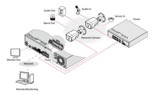
DirectIP™ NVR makes it easy to use cameras without extra network configurations.
