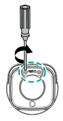
Make sure that the cover is joined properly when screwing it; otherwise, the IP67 level is not guaranteed.
