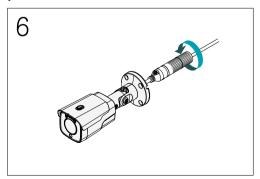
6 Lock the waterproof cap into the waterproof cap body.
