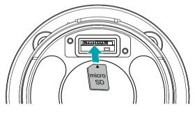
Push the SD memory card until it disengages from the slot, and then pull it out.
