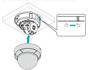
Fasten the screws for the dome cover clockwise using the Allen wrench provided with the camera.
