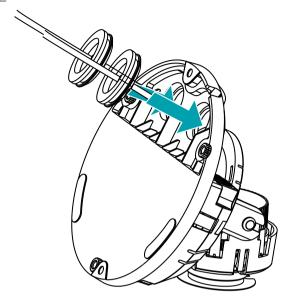
3 Use the screws, anchors provided with the camera to secure the bottom cover on a wall or a ceiling.
