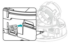
Push the SD memory card until it disengages from the slot, and then pull it out.
