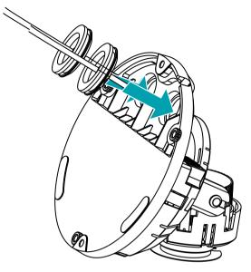
**3** Use the screws, anchors provided with the camera to secure the bottom cover on a wall or a ceiling.
