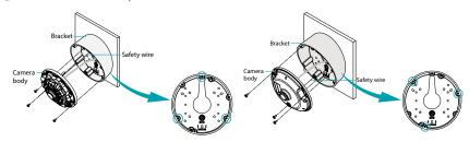
4 Screw the camera dome cover onto the camera body.
