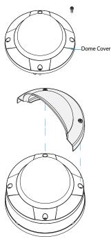
3 The lens of the camera is not covered by the sun shield.
