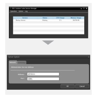
Address, Port: Set up the IP address and port number of the administration or federation server for connection to the administration or federation service.
