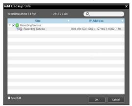
Site: Displays recording services and DVRs that are currently connected to the administration service via the network.
