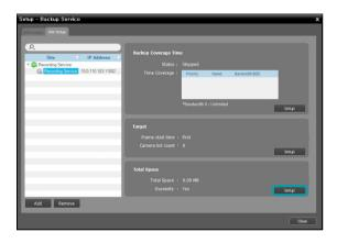
Click the **Total Space** – **Setup** button after adding backup sites and the **Storage Setup** window appears. Click the **Add** button at the bottom. The **Add Storage** window appears, and a list of available hard disk drives is displayed with information about each drive.
