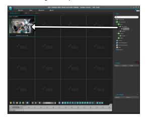
If a layout is registered on the administration service, you can play video in the layout format by selecting a desired layout from the **Layout** list and dragging and dropping it on the Backup Search screen.
