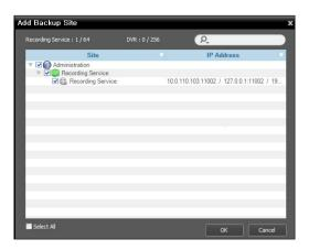
Site: Displays recording services and DVRs that are currently connected to the federation service via the network.
