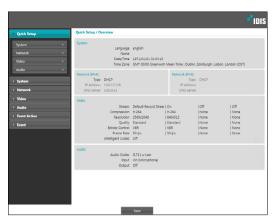
From the Remote Setup screen, select the menu on the left to display the current settings. Select an option under the menu to change the corresponding settings. Once you have changed the settings, click **Save** to apply the settings.
