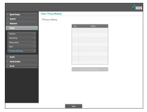
Privacy Masking Setup: Set up privacy masks (up to 8). Privacy masks are set up on Original View video. Thus, if video is dewarped, privacy masks are also dewarped.
