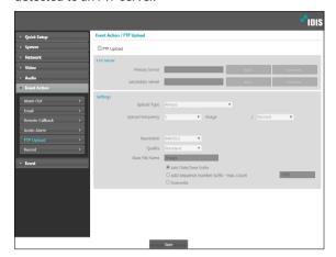
• FTP Server: Click Add to register a new FTP server. Click Remove to remove a registered FTP server. When an event is detected, a .jpg image of the event detected image is uploaded to the Primary Server. If the upload to the Primary Server fails, the file will be uploaded to the Secondary Server. Upload to the Secondary Server will continue to be attempted until successful. Fill out the fields below and click Test to test the FTP server connection settings. Once the test is complete, click OK.
