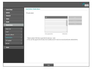
List: Displays a list of audio files to playback. Click Add or Remove to add/remove audio (.wav, .mp3) files. (supports 16-bit, 16KHz encoded files only) Select an audio file from the list and then click Play to listen to the file.
