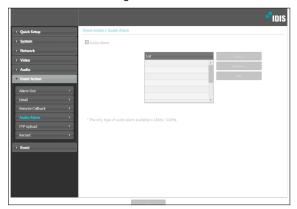
List: Displays a list of audio files to playback. Click Add or Remove to add/remove audio (.wav, files. (supports 16-bit, 16KHz encoded files only) Select an audio file from the list and then click Play to listen to the file.
