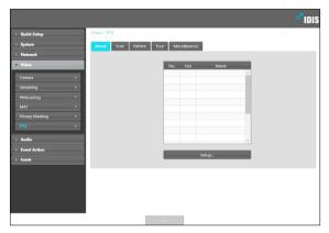
Displays a list of preset. The number indicates the preset number. Click **Setup** button to configure the preset.
