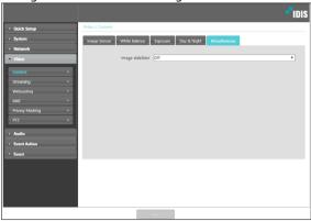
Image Stabilizer: Disable or enable the image stabilizer function. When the image stabilizer is enabled, it reduces blurring caused by camera shake that results from external conditions such as the wind.
