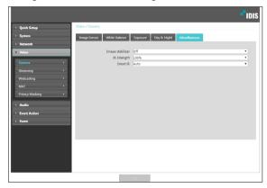
**IR Strength:** Set the brightness of the IR LED. The higher the value is set, the brighter it is.
