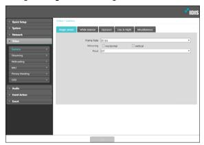
Frame Rate: Set the frame rate of image sensor.
